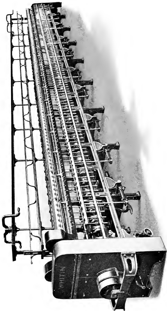
Ring Spinning Frame, with Tape Driven Spindles
